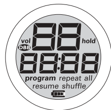
test pattern 2 (alternate segments activated)
